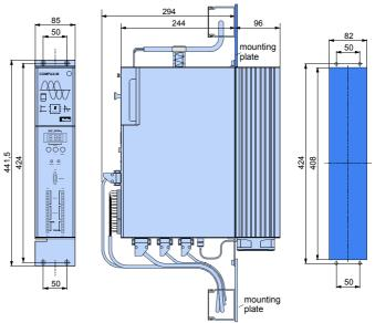
The heat sink is pushed back through a hole in the panel (on right of diagram). A separate heat chamber is created between the installation plate and the rear wall of the control cabinet. The angles required under designation MTS2 must be complied with.
